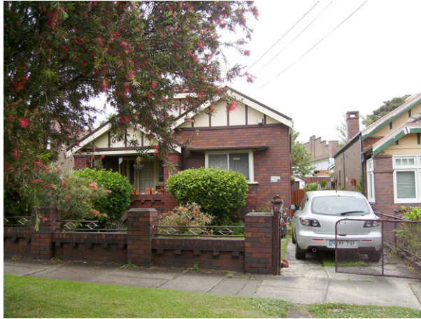
Figure 34.7. Note also the offset of each cottage on its lot to provide access to a side driveway and the simple wire gates divided unevenly to provide a pedestrian and vehicular opening.
