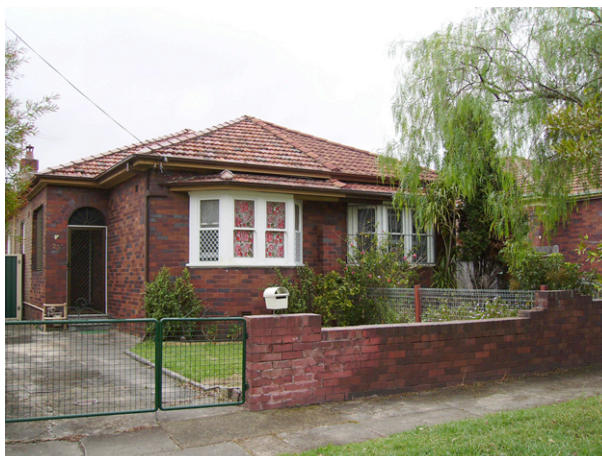
Figure 34.11. The northern side of Stanley Street is characterised by later semi-detached bungalows and small cottages, mostly built in the art deco or austerity style. One of the main differences between the two styles can be seen in the roof form, with the art deco utilising a hipped roof configuration rather than gables.
